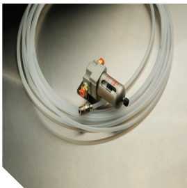
Installation kit (contains 25'1/4" O.D. tubing, in line air filter, 2-1/4" compression fittings, one (1) set of gaskets Part#: VMFPPMIK
